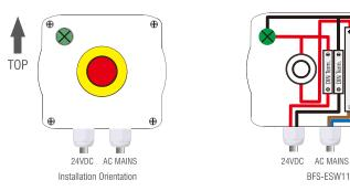
Using appropriate fixings attach the BFS-ESW11 unit vertically to the chosen surface.
