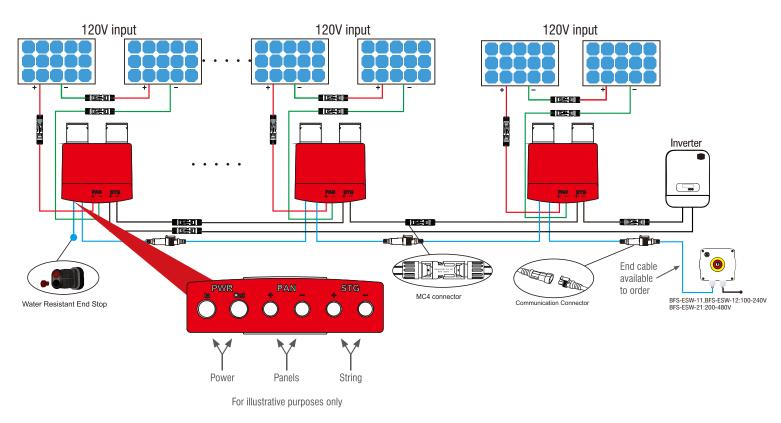
If the array has an odd number of panels, a single panel can be connected directly to the positive (+) and negative (-) panel cables of the BFS.
